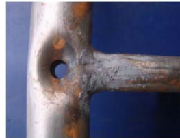
Before and after: A metal furniture manufacturer uses Lab-metal to smooth over rough welds and joints prior to powder coating.
