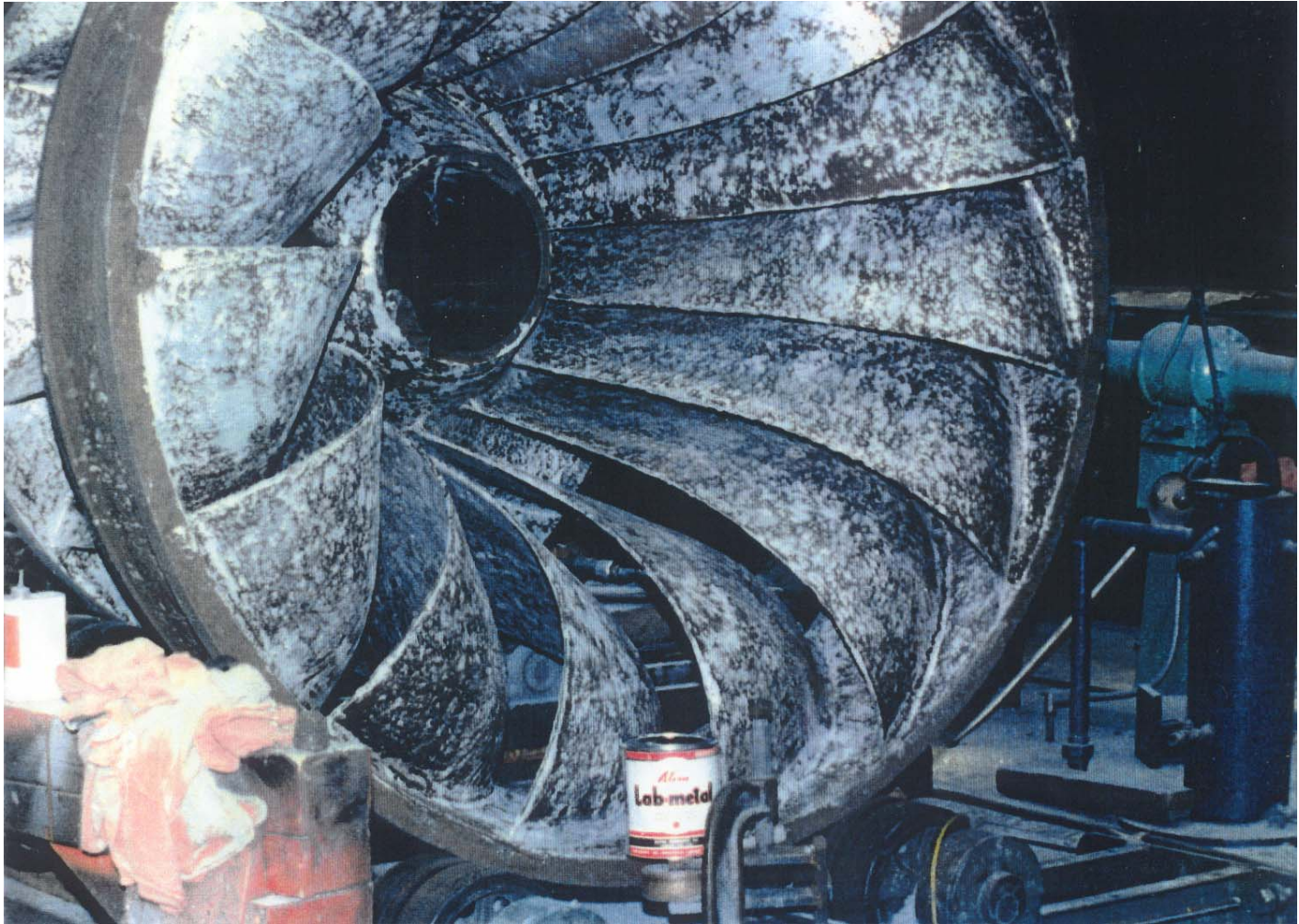
Blades of a Francis Runner (a type of turbine used in power generation ) being resurfaced
