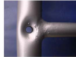
Before and after: A metal furniture manufacturer uses Lab-metal to smooth over rough welds and joints prior to powder coating.
